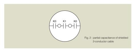
Once the **partial capacitances** are known, **effective capacitance** in actual use can be calculated simply as series-parallel circuit. And this becomes the job done by cable users.
