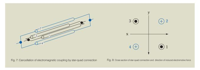
Idea of this method is to short opposite (diagonal) conductors of a four conductor cable to use it as one go and return conductor, considering X-direction of magnetic flux in Fig. 8 cross section, direction of induced electromotive force generated in conductor 1 and 2 loop and that in conductor 3 and 4 are reversed so that both induced electromotive forces are canceld respectively.
